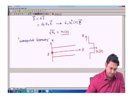
So, the waveguide geometry I need to define for which this condition is valid. So, my waveguide geometry is something like this. So, I have a block like this, this is a known waveguide geometry rather along this axis I say this is my x y axis is perpendicular to the plane and along this direction I have my z the propagation direction. So, the refractive index profile is like a step index profile. So, along this direction I have x. So, it is changing along x direction.
