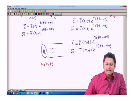
Also it is not restricted with this geometry another kind of geometry is possible which is very important, which is the optical fiber. So, in optical fiber we know that my geometry is something like this. So, the refractive index is changing here. So, my refractive index is a function of r and phi. So, here I can write my electric field in this structure as E as a function of r phi e to the power of i beta z minus omega t and my H as H r phi e to the power of i beta z minus omega t.
