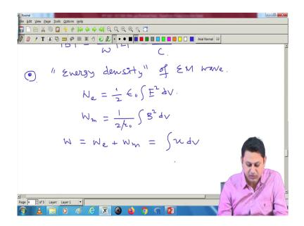
So, we know that the energy in electro electric field we know that the energy can be represented as this. And, for magnetic field also we have an expression similar like this that we know from our basic electrostatic electromagnetic theory. So, the total energy is this plus this and I can write this total energy as the energy density multiplied by the volume, this is integrated over the volume small volume dv.
