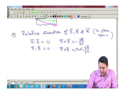
Now, after having the plane wave solution, the next thing important thing quickly we are going to understand is the relative direction of E, B and k. So, three vector quantity we have; so, we are going to find out the relative direction of in free space.
