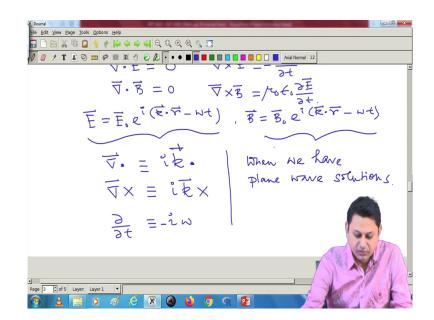
And the solution is E vector is equal to E 0 e to the power of i k dot r minus omega t and similarly I have a solution for B as well. So, B will be equal to B 0 e to the power of i k dot r minus omega t. So, two plane wave solution we have; one is E and another is B. And, now one very important identity, one very important one very important expression that one can extract from the solution is that.
