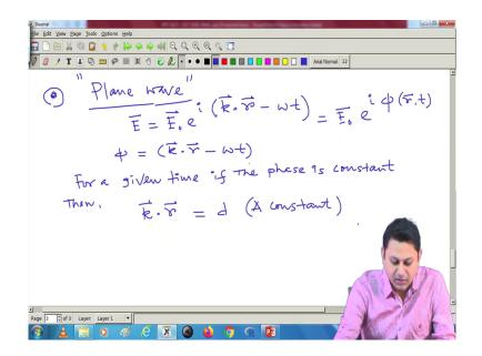
So, quickly we understand what is the meaning of plane wave here. So, I have a solution in this form. So, this is a complex kind of term. So, I can always write this as E 0 vector e to the power of i phi, this thing is scalar quantity and phi is a scalar which is a function of r and t by the way; which is a function of position r and time t.
