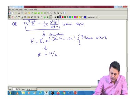
And, for this wave equation I have a solution and the solution is of the form E vector is equal to E 0 e to the power of i k dot r minus omega t. And, when this is solution then there is a relationship between k omega and c and this relation is k is equal to omega divided by c, where k is called the propagation vector. Why it is called plane wave? Why this kind of solution are called plane wave? This is called plane wave by the way, these kind of solutions are called plane wave.
