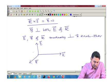
So; that means, that readily means readily tells us that E vector, B vector and k vector mutually perpendicular to each other. That means, if I plot in this direction E then B will be in this direction and k will be in this direction and that is precisely the k is for electromagnetic wave.
