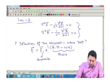
So, let us start quickly. So, today we have lecture 2. So, we have two equation that was the first equation we have the wave equation for electric field. And, also we have the wave equation for magnetic field, these two equation we have. So, today we will try to find out the solution and the solution we will find this way; so, the solution of the Maxwell's wave equation.
