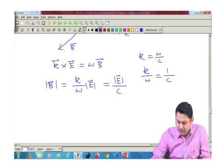
So, I have curl cross E k cross E is equal to B omega. So, I have k cross E equal to omega of B. So, if I want to find out the magnitude of B, it should be k divided by omega and then the magnitude of E and now we have a relation between k omega and c. So, k is equal to omega divided by c.
