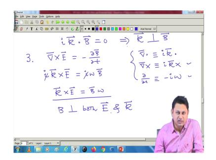
So, k is perpendicular to B and E both fine, then we will going to use my 3rd Maxwell's equation which is the relationship between E and B. So, curl of E is equal to minus of del B del t, again I can replace this curl operator because let me write it once again. So, whenever I have this, this is equivalent to i k dot, whenever I have curl is equivalent to ik curl, whenever I have del del t this is equivalent to minus of i omega.
