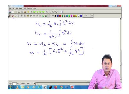
So, from this three equation you can really find out the energy density is simply half of, the energy density means the energy stored in a EM wave, energy stored per unit volume. So, this quantity is simply half of epsilon 0 E square plus 1 by mu 0 B square this.
