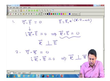
So, we will going to make use of that to all the four equations, we have four Maxwell's equations. So, first equations I have grad dot E equal to 0. And I know the solution of that E
