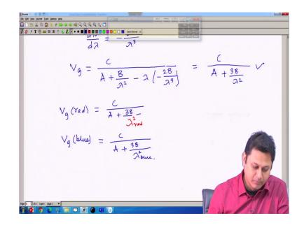
Now, if I calculate for red so, V g for red will be C divided by A plus 3B divided by lambda red square and maybe I can write this in a. So, this lambda square because since this is a red. So, I can write it in this way. And V g blue is C divided by A plus 3B divided by lambda square blue.
