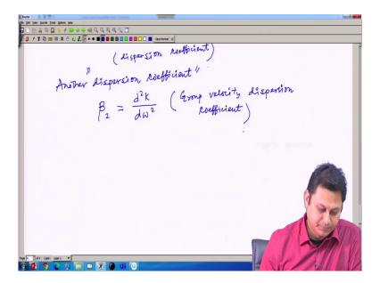
So, another dispersion coefficient ok, which we defined as beta 2. This is standard notation to define a dispersion coefficient beta 2, which is by definition d 2 k d omega square and is called the group velocity dispersion coefficient.
