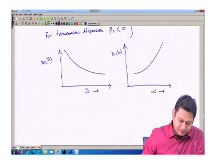
So, let me try it out. So, this is if the curve of dispersion the refractive index as a function of lambda and this curve is drawn in a normal dispersion regime when the refractive index is changing with respect to lambda and decreasing. So, when the refractive index is decreasing with respect to lambda then it is in normal dispersion and when it is increasing with respect to lambda, then it is an anomalous dispersion.
