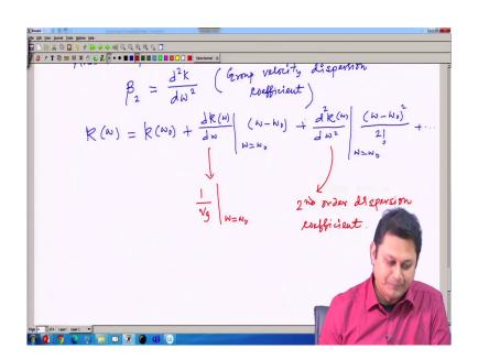
Now, one can realize this coefficient by expanding the propagation constant k as a Taylor series, which is a function of omega. See if I expand around the wavelength around the frequency omega 0 this is the operating frequency. So, it should be this evaluated at omega equal to omega 0 and so on.
