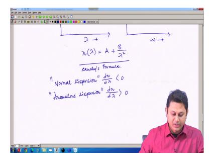
So, this equation follows the Cauchy's relation. So, if I write the Cauchy's relation side by side it should be this equation is following this. So, it is very much in normal dispersion regime, this Cauchy's formula. Now, for normal dispersion as I mentioned we have d n d lambda is less than 0 and anomalous dispersion it is d n d lambda greater than 0.
