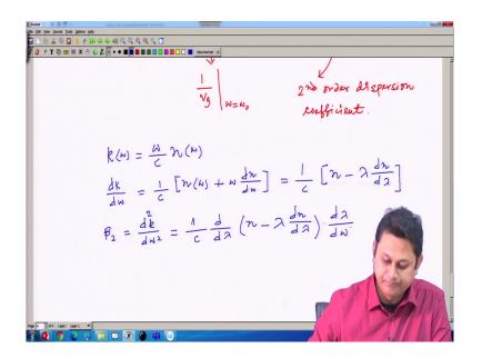
Now, if I want to find out the value of beta 2, we can do that because I know what is the expression of k, because k omega is omega divided by C n of omega. d k d omega I can calculate which we have already calculated. This is 1 by C n of omega plus omega d n d omega in terms of omega. In terms of lambda it is 1 by C n minus lambda d n d lambda in last class we have already calculated that.
