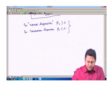
Now, for normal dispersion when the refractive index is increasing with respect to frequency that we call the normal dispersion. So, for normal dispersion we have beta 2 greater than 0 and for anomalous dispersion, this is another thing called anomalous dispersion beta 2 is less than 0.
