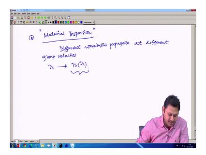
After, that we will directly jump to one of the major property of waveguide, which is called the material dispersion, material dispersion. So, quickly we brush up the material concept of material dispersion. So, different wavelength is nothing but the different wavelength propagates at different group velocities. So, different wavelength propagate at different so, that happens because n is a function of lambda. So, that is the main issue here. So, the refractive index n is a function of lambda.
