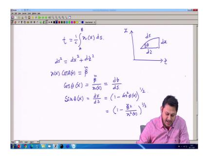
Well, now my t, as I mentioned should be simply integration of 1 by c because c is a constant should be come outside n X d s, that integration from one point to another point say point A to point B, I need to calculate. This is this should be the recipe to calculate the time. Now, d s square I can modify slightly. This expression is equal to dX square plus dz square because this is the structure. So, let me draw this side so that this is dz, this is dx, ds, this angle is theta.
