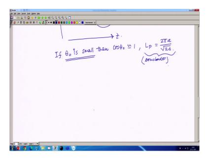
If theta 0 is small, then we can, we can say cos theta 0 is nearly equal to 1 and for that, I have L p is equal to 2 pi a whole divided by root over of 2 delta and that is independent of that is almost that is constant and independent of if any theta 0. So, we can have all the, all the ray is in the same period, but with the condition that this has to be theta has to be small; this is the condition, theta is small. This is a specific condition under which we have this, ok.
