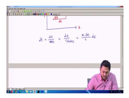
Now, dt will be ds divided by v of X. d t is the time that should take the ray going from this point to this point. In order to travel the ds path, what is the time taken by the ray is d t here. Now, this quantity is d s divided by c n x or is simply n of x divided by c ds. So, I need to evaluate this right hand side, in order to find what is the value of t, the entire time.
