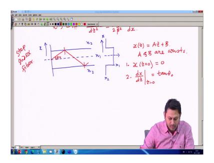
Now, if I have a fiber structure like this, refractive index n 1, n 2, n 2 and it is a step index kind of fiber. This is n 1, this is n 2, this is along x. Now, for this structure, if I launch a light, it should follow a straight-line path. If this is my launching angle theta 0, we calculate using the ray equation, we calculate the path follow a general equation should be AZ plus B; where, A and B are constants, where A and B are constants and can be evaluated using the boundary condition.
