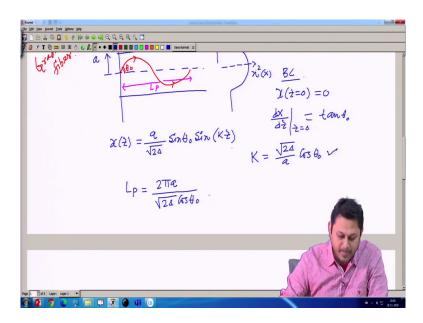
And the value of the K, that we calculated last time was root over of 2 delta divided by a and cos theta 0 that was the value of K depending on the initial angle theta 0, depending on the initial angle theta 0. Now, also we calculated the period; once we know what is K, then we also calculated the period and L p was the period, where L p is this amount. From this, this is
