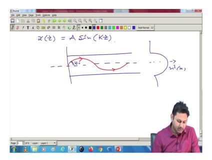
So, I simply have x is some constant A sin of K Z. So, it is simply a sinusoidal wave, if I launch, if I launch this wave exactly at this point for a parabolic structure, then it should follow a sinusoidal path. A very interesting thing that I find, for step index fiber it was a straight line, but in parabolic index profile, this is a parabolic index profile. So, the path it will going to follow is sinusoidal in nature.
