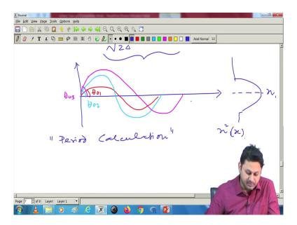
So, let me draw finally, how the path will look like for a parabolic? So, I need to draw this drawing is slightly I need to make it better. So, this is the profile I have and here at this point I have n 1. So, this profile is this is a n 1 square x profile, parabolic profile and the path the ray will follow is this. This is one path that I follow, another path let me draw it another line, and another path it can follow something like this.
