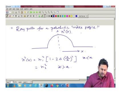
However, today we will going to find the ray path for a parabolic index profile. This parabolic index profile is not new I already introduced this in one of the classes, previous classes and the profile looks like this. Along this direction it is suppose n square x this is the direction of X. And, mathematically it was n square X is equal to n 1 square 1 minus 2 of delta x divided by a whole square for this region.
