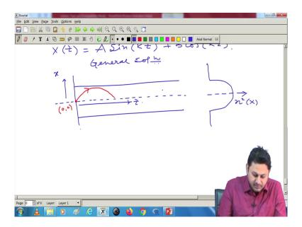
Again, I will going to draw the structure. And, here the profile, this is a parabolic profile. So, this is n square as a function of X and along this direction I have my x, and along this direction I have Z. Since, it is a sinusoidal kind of wave, I can launch the wave exactly at this point and if I launch here it should follow a path like this. Now, note it here I launch at this stuff at 0, 0 point. So, this point is 0, 0 at origin.
