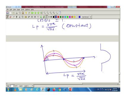
So, under such condition what happened, all the rays will follow the same period. So, for small launching angle so, I can write it, I can draw this in this way. This is one ray for nearly
