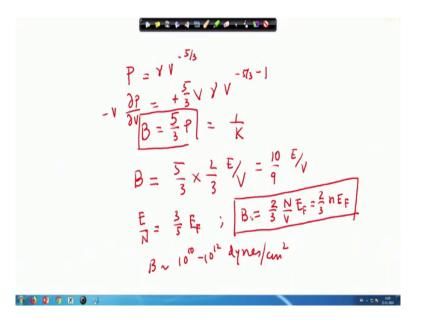
Now, again I go back I just derive the fact that P is some constant times V to the power minus 5 by 3. So, V to the power minus there; so, all I have do is to take a derivative of del P del V
