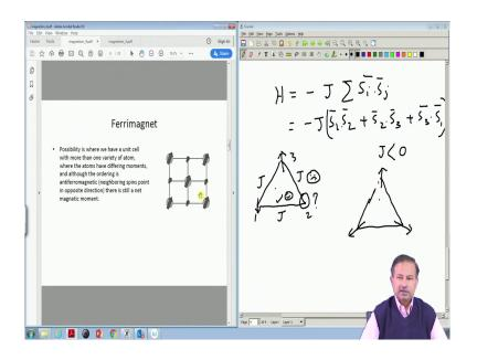
Then of course, I discussed ferrimagnet at some point where you have usually two different atoms in the neighbor. And so, their spins have different magnitude, their moments have different magnitude, and this alignment is kind of alignment is called a ferri magnetic alignment ok.
