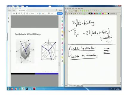
So, this is the tight bind tight binding, in tight binding approximation you saw that for the square lattice. For example, E is a minus 2 t cosine K x plus cosine K y E of K E of K. Now, this is a again set episode not equal 0 this is the simplest.
