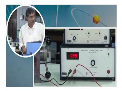
now if I give if I apply current, if I apply current ok; if I apply current some 1 point, say 1 ampere current I applied and now field we noted down the field, it is 1254 ok.
