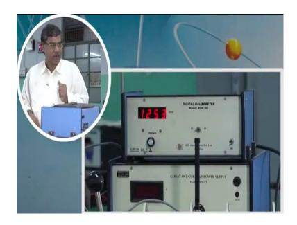
then we increase the field; increase the current to 1 point say 3; 1.3 then it is the field is increasing current versus magnetic field current versus magnetic field, we can note down and we can plot and from that plot you can find out a slope. that is the calibration of this electromagnet with current ok.
