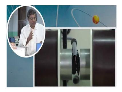
this is the probe and this probe connected with this meter. as a whole these are gaussmeter.
