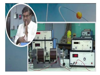
this as I told that when you come in the lab teaching laboratory we will see that there is a magnet and there is a probe. Now, probe is put inside the between the pole gap and there we want to where we want to measure the magnetic field ok.
