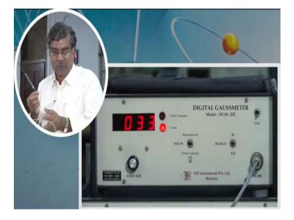
And that constant is divided this the v voltage is divided by that constant through the electronics and whatever the value that is shown here. that is reading of the magnetic field ok.
