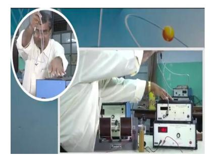
this is probe you know. just let me open it. this is probe this is probe and this is the meter this together is we tell the hall probe or gaussmeter or teslameter ok.
