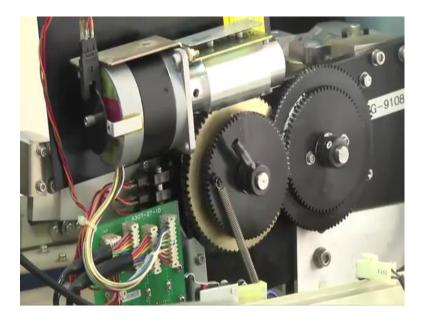
That that stepper motor that is also standard that stepper motor is connected with this detector holder and from computer programming one can choose the step of this change of the angle 2 theta or change of the angle of the detector and from 0 to 90 degree, we scan and on screen, we will get the X-ray diffraction pattern.
