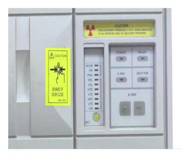
Here you can see that and in here, it is written power then X-ray shutter on off. from outside itself, we can see whether X-ray is on or not whether it is a X-ray is produced. Some shutter is there we just can close the close the exit of the X-ray using the shutter.
