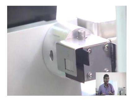
This is a detector. It is the X-ray detector if it can measure the intensity of the x ray. As I for any detector, in this case, X-ray will fall and then it will produce equivalent number
