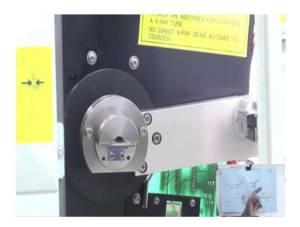
it is a door I will open it this door if I open this door and I will open this backside also to show you to show you just I can open it. Here you can see, when I open door immediately I am able to see here, we put sample we put sample this is the sample holder
