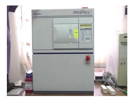
Here you can see this is the machine, we tell this X-ray machine and it is X-ray diffractometer.
