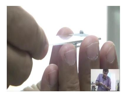
This you can see powder this is the sample powder, we put slight amount of powder on this on this. just paste it spread over it. The sample that sample now I will put in sample holder I will put in sample holder here I am putting now, sample is there. Now, here you can see here there is an X-ray generator; X-ray generator here I will show you from backside. From this X-ray generator this X-ray will come and there is a filter inside.
