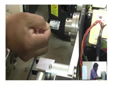
This sample here I have put sample. this powder sample soon a glass plate. You put in the sample holder. Now, this is fixed, but the detector this is the detector X-ray detector, which can detect the intensity of X-rays. This is on this liver on this arm. this arm you can see this is the free to move free to move from 0 degree to 90 degree.
