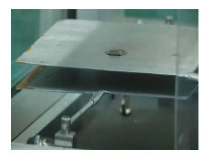
This is one top one it is the movable and the bottom a one bottom one that is the fixed this same as these 2 conductor parallel conductor now that is the replaced by 2 capacitor plate ok, bottom plate is fixed top plate is on the lever so it can oscillate.
