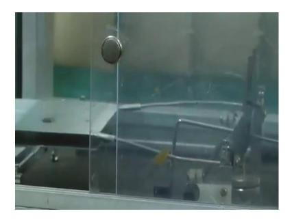
This lever here you can see this that is the lever axis and that is the mirror. This capacitor place from the middle we will take this distance small a now I have to measure force for different voltage in this case for different voltage. Now here one difference is that other case I was initially, I was what is the position of the laser spot that I marked.
