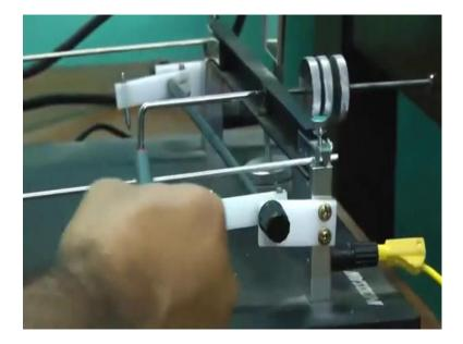
current is coming now this is conductor top conductor current is flowing this way and going back here and then coming through this black wire and here and then the conductor below current is going this direction and going back to that source current on top one current will go in this direction and bottom one current will go the other detection so there will be repulsion. Now I will apply current and, I will take it back to the original position.
