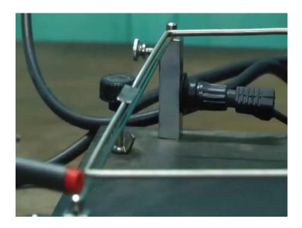
And, another conductor is below this is fixed below you can see this the another conductor, this is fixed and with respect to this top one see it is on this lever so it can change the position ok, it can change the position. Now just for a particular separation, for a particular separation for this particular separation I want to measure this separation d 0 as I told because I will do experiment at this for this length of this wire capital L.
