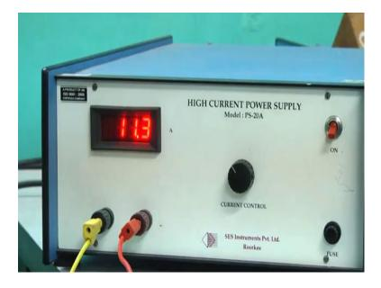
Here I will switch on this magnet, this not magnet this power supply it is a high current power supply because current generally for this mass we have to apply around 10 ampere current. now, I will apply current as long as this laser spot will go back to this original positions and how much current I have to apply. Now I will apply the current here you can see I am applying current.
