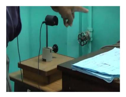
We are using to get that one we are using laser, you see this is a laser now this laser light is falling on the mirror, here you can see this one mirror this laser light fallen on it. this mirror, so this mirror is fixed on this on the lever with respect to; with respect to that lever so these are rotating these are rotating ok, these are rotating.
