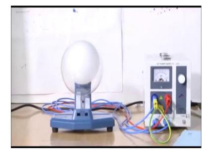
This is a simple setup for Electron Diffraction. this it is a cathode ray tube, cathode ray CRO tube And with this CRO tube this spherical this ball kind of ball, this is the whole system is in vacuum this one can think of that it is a skin since CRO cathode oscilloscope the same types of tubes are used electron beams are coming and falling on the skin. Here this part white part we will use as a skin.
