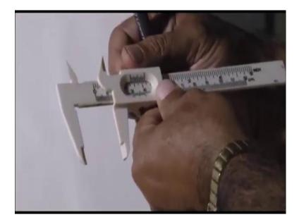
it is Vernier constant is for this 0.1 millimeters, 0.1 millimeter 0.01 centimeter ok, yeah yes 1 by 10. I think this is the very elementary I have discussed ah this one in experimental physics so on, how to find out the Vernier constant I will use for this first ring whatever the diameters outer diameter and inner diameter I have to measure for second thing also same way I have to measure. Now, you see just see table experimental data experimental data ok.
