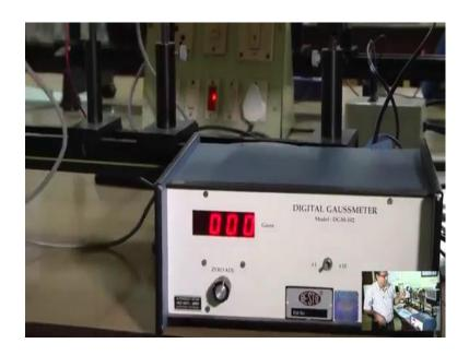
This is the gaussmeter, it has a probe. It will give me reading initially, now, it is reading is 0 Because, I have not applied any current or it is away from that magnet ok.
