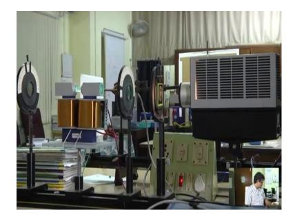
This is the experimental set up here, we have arranged this experiment. As I told this there are two components main components in this experiment; one is light, another is magnetic field.
