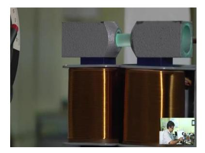
Here will fall on the sample, this is the sample here this is the sample between two pole pieces of bar magnet because we have to apply magnetic field. for the magnetic field what is the arrangement that I will tell you, but before that let me finish that light will fall on the sample and pass through the sample and that light then it will fall on the another polarizer. We tell this is the analyzer polarizer and analyzer are same. It will fall on this analyzer ok.
