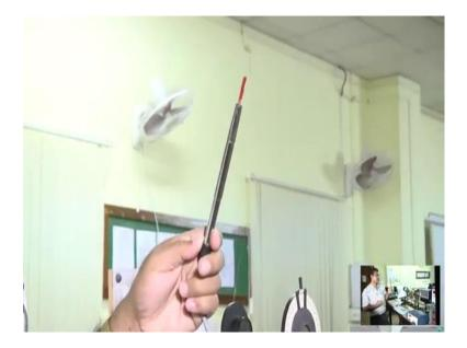
Now here this is it is the hall probe; I will in separate class, I will when I will discuss basic tools and instrument in a laboratory during that time I will discuss about the principle of this hall probe. Here this probe a transverse probe here magnetic field if we want to measure between two pole pieces I have to apply like this.
