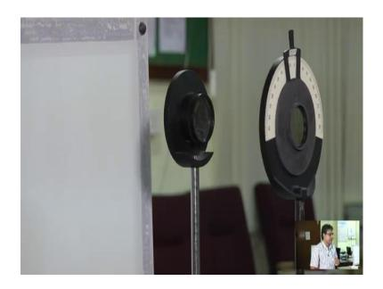
Here we have used one lens and this is the screen. One can use also photo detector to see the intensity of light. We have to measure the intensity of light. Here we have used one lens and then this is the screen on the screen you will see the spot of the light coming.
