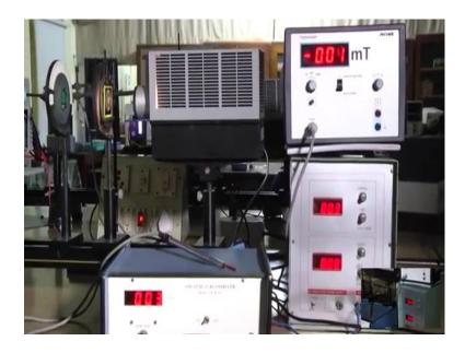
This is the power supply; this is the power supply for constant current power supply. Here you can see is the, here we can change the voltage and here we can get the current. If we change the voltage then current will vary. We will set at a particular current and for that current what is the magnetic field between these two pole pieces, where we have kept the sample or we will keep the sample that we have to note down.
