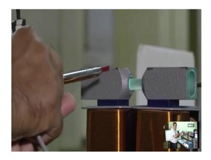
Perpendicular to the axis of the pole piece, I have to apply this this way. That is why it is a called transverse mode ok, transverse probe. In addition, but here we want to magnetic field along the axis and inside the you see sample also it is inside the pole I cannot put here inside this way. I have to put this one like this along the axis I have to measure the magnetic field for that this is the special type of pole pieces there is a hole between that inside these pole pieces.
