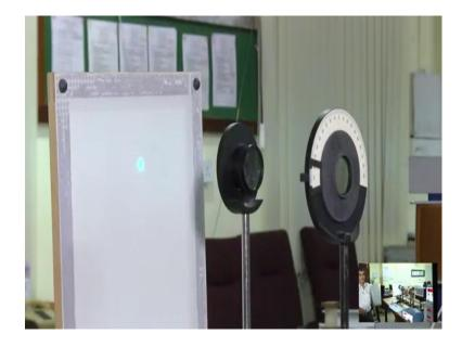
If I maximize this green this intensity of the green speed spot I will rotate it I have to make it if both are aligned so intensity. It should be also near the 90 degree what is the value now? It is at 90 degree it is at 90 degree, you see this is at 90 degree that is also at 90 degree intensity here spot you are seeing this is spot as I told polarize light. Now without changing the angle of polarization it is falling on the analyser; all light passing through it ok.
