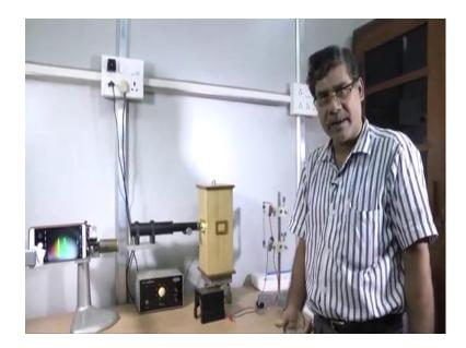
Now I will demonstrate you how to measure the wavelength of unknown light using the constant deviation spectrometer. this is the setup for the constant deviation spectrometer, as I showed you in the schematic diagram; that this is a source this is a source. Here we are using I think this is mercury source. one of the line we will use as a known source known wavelength ok.
