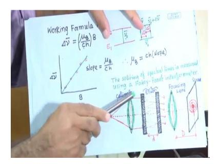
This is the etalon as I showed you as I showed you here ok. now, in front of this there is a lens here collimator lens. It is here and the other side also another lens is there another lens is there inside you cannot see. This together is it is the interferometer ok.
