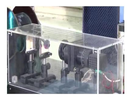
For that, we have used this interference filter. This interference filter it will just allow to pass this green light of having wavelength 546. In addition, with some bandwidth with some bandwidth of course, and other light will not pass through it.
