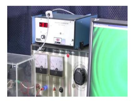
This is the power supply for the electromagnet. There are 2 coils. in that coils we pass current; here you can see current and voltage it is a one can see. We give we pass current through these coils and then, it will produce a magnetic field. magnetic field will vary with current.
