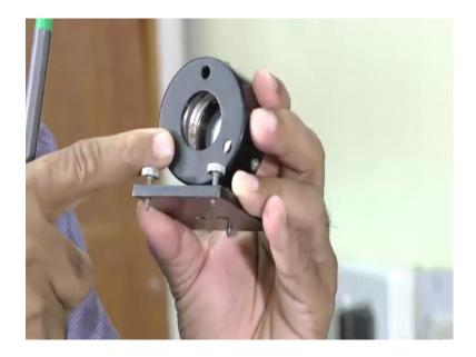
In addition, other side you can see this is another mirror. One mirror is fixed another mirror you can adjust with this screw systems are there, here 3 screw systems are there. You can change the adjust the distance of this of these 2 mirrors. Or you can also tilt it you can adjust these 2 mirror. This type of things we have used here. this in front of that one there is a lens as this type of setup ok.
