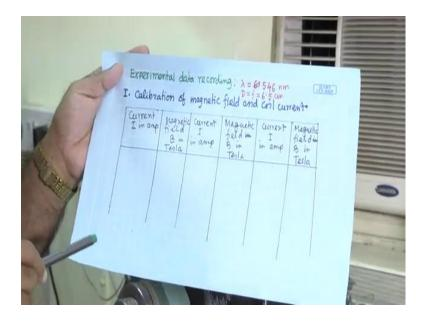
Calibration of magnetic field and coil current it amperes or milli amperes and then corresponding magnetic field using the Gauss meter, ok.
