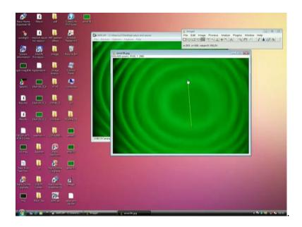
This would be the diameter ok. Diameter of this of this ring first ring in pixel, you will get from this software or you can take print out and then all alone can use scale and pencil to find out the diameter. that you have to for first ring for second ring third ring.
