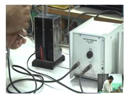
This is the frequency from here the frequency ok. This frequency meter it is generating this it has a RF oscillation and that RF oscillation we will put from here this tank circuit inside there is an induction coil.
