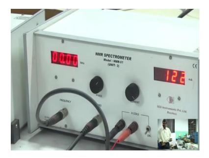
You can see here is retained NMR spectrometers. in this experiment as I told that, you need sample to put in the permanent magnet between in the constant magnetic field produced by a permanent magnet and that Helmholtz coil to a pair of Helmholtz coil will be pair of Helmholtz coil will be attached with this permanent magnet from where AC field will be modulated with the permanent magnetic field constant magnetic field.
