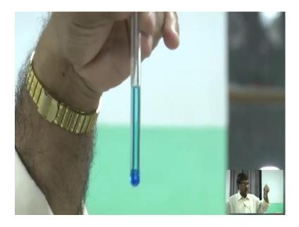
Here you see this is our sample is a copper sulphate is the copper sulphate solution. this nuclear of nucleus of this copper have here spin half ok. This sample is used.
