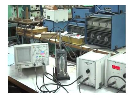
This is the experimental setup or of NMR spectrometer.
