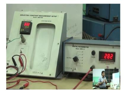
Here different scales are there whatever reading you will see we have to multiply with this one. this pico ampere into this reading. Different range one can choose. now so this is for as I showed you this circuit is made here, this circuit is made here it is a simple circuit. Now we need arrangement now we need arrangement heating arrangement this green wire whatever you are seeing that is thermocouple it is connected close to the sample.
