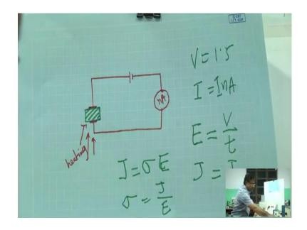
You should have provision to heat the sample and measure the temperature. for that you need arrangement as well as you just this is the simple circuit diagram. You have applied a constant voltage and what are the is the is the current flowing through this circuit. That we will known the from this nanoammeter or picoammeter in this case here we are using picoammeter. Naturally you can see this very small change of the very small change of the current we have to we have to determine.
