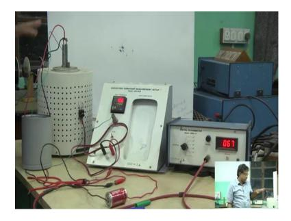
This is the experimental setup for ionic conductivity measurement and for determination of the activation energy. As I told that this measurement is, very simple it is an Ohms law experiment circuit diagram is just here you can see this is your sample ok.
