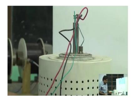
Now, this furnace kind of things hole is there. I will insert this one through this hole now; my sample is in oven; and for protection for less heat radiation to reduce the heat radiation.
