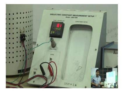
Oven is off it is up its off when I will put down so this it will start heating. This is the oven so it is this is the power supply of the oven and temperature controller. Through this through this, it is the power to the heater is given so heater here inside heater is there. Power from here the is given to the heater.
