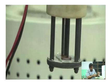
So let us see my sample here I can show you our sample. I think it is a slightly hot this you see this tablet rather sample here this a tablet kind of sample this is the sample. Thickness of this tablet it is the plate thickness of the plate and radius or diameter of the plate is known it is supplied or one can measure also.
