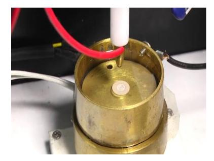
We have used this silicon oil for uniform heating of the sample. Here this is one electrode; this is one electrode, this falling on top of the sample top of the sample and bottom of the sample on this platform. It must be isolated from this other parts other part.
