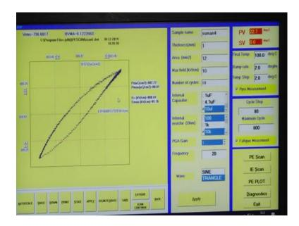
I asked for P-E loop between this maximum fields 10 kilovolt per centimeter, it will take 10 number of cycles, and take the each cycle it is varying the it is varying the electric field ok.
