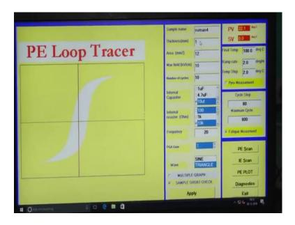
In computer all information is given here, you can see here you can see that thickness of the sample is 1 millimeter that we have to give information to the computer. What is the thickness of my sample? This is 1 millimeter what is the area of my sample? This is 12 millimeter. What is the variation of the field I want?
