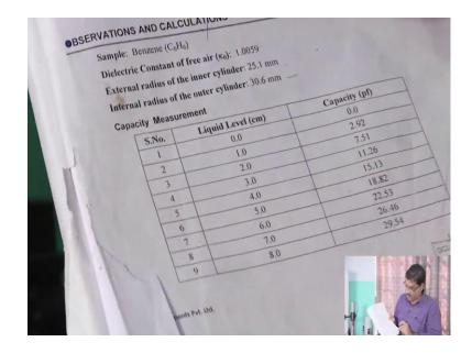
Now, we will get this you see that dielectric constant of free air 1.0059. External radii of the inner cylinder 25.1 millimeter; internal radii of the outer cylinder 30.6 millimeters; this is the parameter is given, so using that parameter now at different liquid level we are we have noted down the capacitor.
