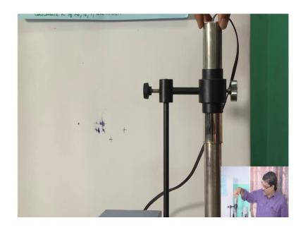
I think; so this one is power supply as well as the this the capacitance, We are measuring it is connected with this capacitance meter, nothing needs to show you here because inside that capacitor I cannot show you because this the compact system only we have very nice, this very simple and we have very nice option to change the height of the liquid or level of the liquid and directly we can get the reading from simple capacitance meter. I think I will stop here.
