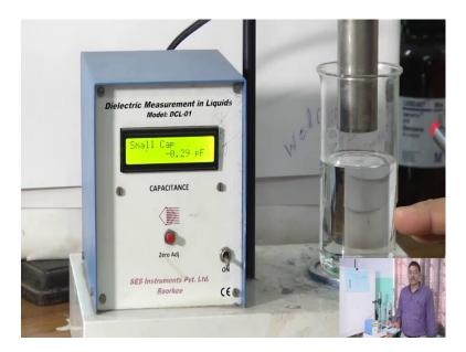
Measurement of dielectric constant of non-conducting liquid.
