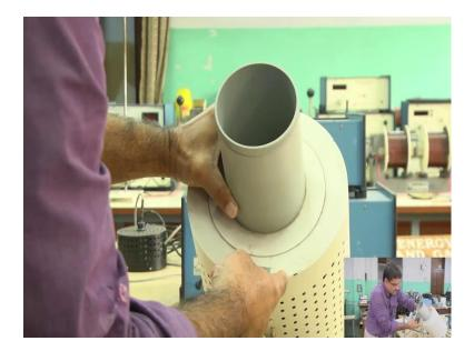
This is oven. You can see it is an oven inside ceramic hole is there this is the oven this outside, outside in this inside is box. Outside of this ceramic tube there are coils heating coils ok.
