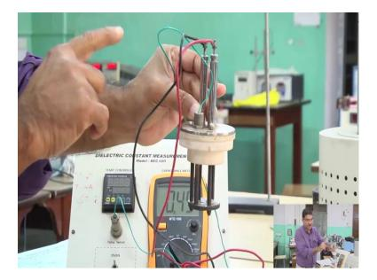
Now we will apply power and here you can see three connection this two for applying electric field as well as for measuring the corresponding capacitance. In addition, these blue line; this one is a temperature sensor, is a thermocouple it is inside this. inside thermocouple is there. This through this wire, we will get the temperature this we will put into this oven. We will put into this oven. I have to put carefully. Yes, I have put
