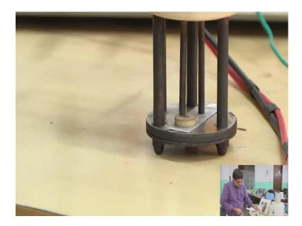
Here you see in bottom, there is a metal plate in bottom that tablet is put on a bottom. I think yes this is isolated from this base using the mica foil for electrically isolated. Only
