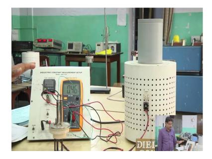
This is the experimental setup for measuring the dielectric constant of a solid. Here you can see this in our sample; this is the sample it is a tablet kind of things looks like tablet ok.
