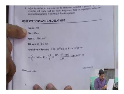
Then you are getting then as I told it is a we have to know the dimension of the we have to know the dimension of this material. here diameter is 9.97 millimeter. company has supplied this sample as well as this diameter one can measure also. Corresponding area will be this. In addition, thickness of the sample, that is an important that is 2.45 millimeter. In addition, epsilon 0 is this one 8.85 into 10 to the power minus 12 farad per meter.
