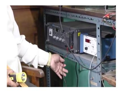
Electromagnet for power supply here; power supply here. we are applying current to the coil of the electromagnet from this power supply. This DC power supply. and this is the gauss meters This is the Hall probe; this is the Hall probe; Hall probe.
