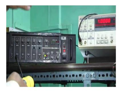
that I have put to the amplifier of the loudspeaker. loud speaker will vibrate with this same frequency of the signal of the signal and the, what about amplitude we have given that amplitude I can amplify here. 80 hertz signal sinusoidal signal here you can see these which type of signal. It is a v 10 anyway.
