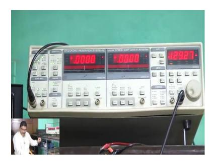
This one is amplifier; lock-in amplifier. this signal whatever we are getting from the sample, we are getting from the pickup coil, that signal we have giving to the input of the input of the lock-in amplifier.
