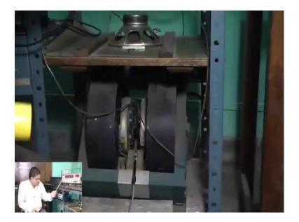
I can show this is the electromagnet and this pole piece these two are pole pieces. These two are pole pieces electromagnet that, we have power supply here.
