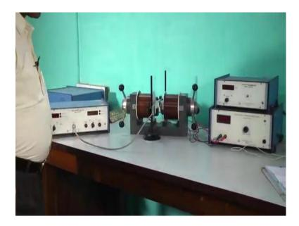
this is the experimental setup for Hall effect. earlier setup whatever I have shown you; here also same setup only we have provision for changing the temperature of the sample except that one rest of the part here they are same in compared to the earlier setup.
