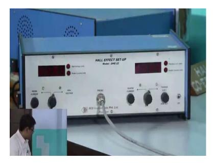
this is the box you are seeing, this box everything giving this power is given from this box to the probe, alit is measuring the temperature as well as the Hall voltage. basically we have here inside, inside the box what we have? Here you can see there is a heater current.
