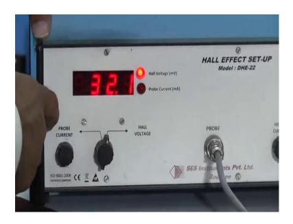
As well as there are 4 connections for the Hall measurement, 2 for current and 2 for measuring Hall voltage. from here there should be 8 connections, 4 for Hall and 4 for heater and thermocouple. I think I will stop. it is decreasing, temperature is increasing. What is the temperature now? 2.98, 2.98 2.98; it's a 2.98 2.97 I can see here; temperature is 73.
