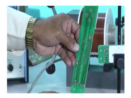
you see from here this connection here is connection PCB. these two connections are coming from the heaters; these two connections are for heater. This last two coming from this two, this is for heater, this is for heater. current is going to the coil it is heating. Now, these two are for the thermocouple; these two are for the thermocouple. here you can see these two are for the thermocouple; these two are for the thermocouple. Here these and these and these for thermocouple.
