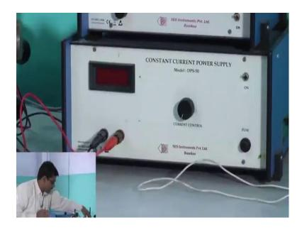
And, this is the constant current power supply for the electromagnet for this coil of electromagnet. And, then we have to; we have to; we have to calibrate the electromagnet for different coil current. we have to for a particular year gap we have to measure the; we have to measure the; we have to measure the; we have to measure the magnetic field using the Gauss meters and Hall probe.
