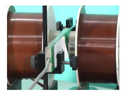
here you can see these we have a sample; we have a sample we have placed the sample between the pole pieces of the electromagnet, because Hall effect magnetic field is compulsory. And, here we have taken sample p type germanium as I mentioned that, if you have p type semiconductor then a Hall coefficient you will get Hall coefficient inversion as a function of temperature means Hall coefficient will have two contributions.
