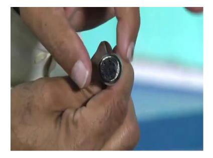
we can see this hole; this is the female type this is the female type hole. all wire is connected inside female type hole.
