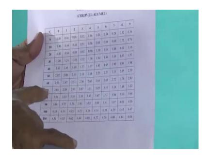
which thermocouple here? company is telling that chromel-alumel thermocouple. at different temperature is produced different thermo E.M.F. here temperature is given in degree centigrade. 0 degree centigrade this 0 value. 1 degree this is 0.04.
