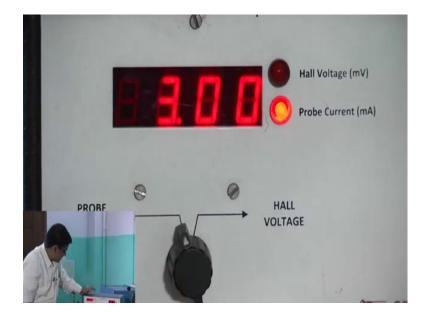
now I am setting say particular current it is in millivolt milliampere, milliampere here you can see. 1 milliampere let me set; let me set 3 milliampere, let me set 3 milliampere current, probe current, sample current that is electromagnet coil current.
