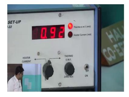
I will set at; I have set at 0.92. as per calibration what is the present temperature? that value here thermo E.M.F. we are expecting 0.92. I have set; slight change sometimes it is there, but does not matter much 0.92. Now, I have to note down I have to note down at thermo E.M.F. is 0.92 corresponding temperature from the chart, it is 23 degree centigrade. And, for that this what is the Hall voltage? 47.8. Now I will change the temperature; I will change the temperature.
