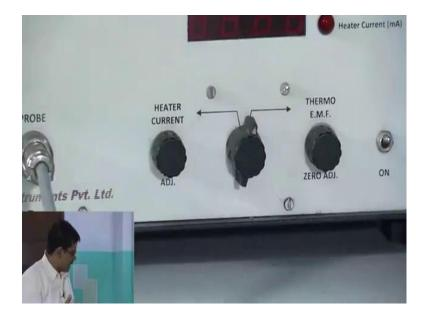
heater means you know this there is a coil of some probably this we use tungsten. if you pass current through this coil, then coil will supply heat and for you have provision to change the heat applying current more current if you apply; heat will be more and temperature will be higher. as I told that we will measure the temperature with thermocouple, I will explain what it is. basically thermocouple gives the E.M.F., it is called thermo E.M.F. and this thermo E.M.F. is the basically voltage.
