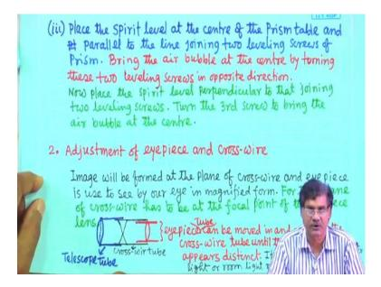
Opposite direction means if one is clockwise, other one would be anticlockwise. Its height of this one side is increasing, height of the other side will decrease. because for leveling it is put in parallel to this two screw, to bring the air bubble at the center, it is necessary if it will be necessary to increase the height of one corner means we are using one screw. Definitely this other side it has to be opposite. That is how we tell rotate them in opposite direction.
