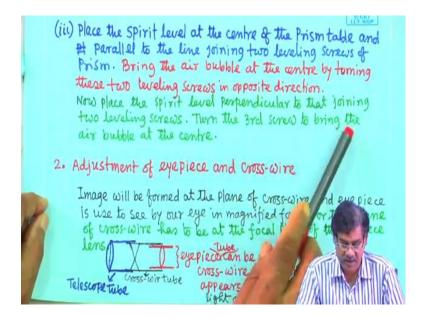
And then you will place the spirit level at the centre of the prism table. And in prism table there are 3 leveling screw. Spirit level you put in such a way that it will be parallel to the line joining two leveling screws. Now, to bring the air bubble at the centre of the spirit level, turn these two screw these two screw this which are parallel to the spirit level in this screw you rotate it in opposite direction.
