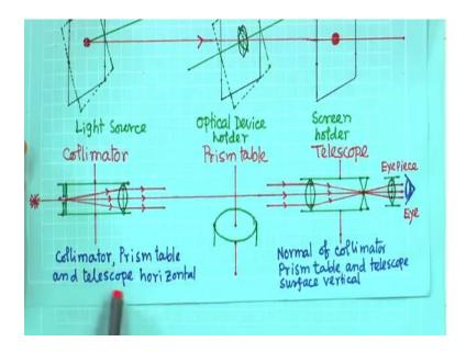
Vernier here you can see if this source of light source say this is on this on this plane, there is a hole here on this plane there is hole. Light is coming through the hole, Vernier this hole acting as a as a source. Now, if light is coming, Vernier small hole is there. Light is coming through it. Now, if this screen is not is not say vertical this way, if it is rotated if it is rotated, then what will happen, light will go along this direction. it will not go in this direction.
