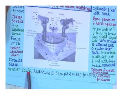
Vernier scale, adjustable slit for height and width for the source, then collimator fixed with base, base stands on. There is a collimator. Collimator fixed with base. There is a base, which base stands on 3 leveling screw. Then prism table with 3 leveling screw and height adjustment and its height is adjustable. Collimator then prism table and then telescope.
