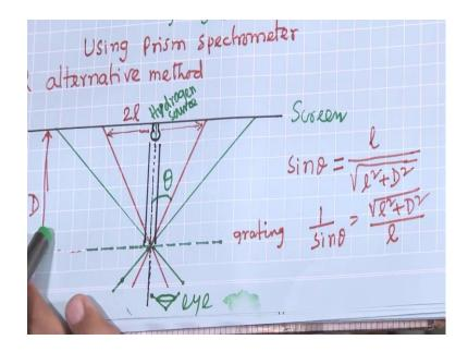
Because here I have written 1 by lambda because in Rydberg constant theirs 1 by lambda equal to R H; as I showed 1 by lambda equal to R H 1 by m square minus 1 by n square. this n is different than the that n that is the order of the diffraction order, but here this n is principle quantum number. from that measurement from that measurement you can get the 1 by lambda using the grating you can get 1 by lambda.
