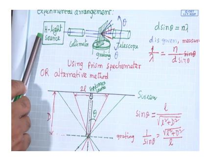
what is the experimental arrangement for this experiment? Experimental arrangement for this experiments it's a, so to measure the wavelength to measure the wavelength of a light prism spectrometer is very popular. in spectrometer in prism spectrometer we put grating on the prism table and then there is a collimators in front of collimator there is a there should be source of hydrogen light.
