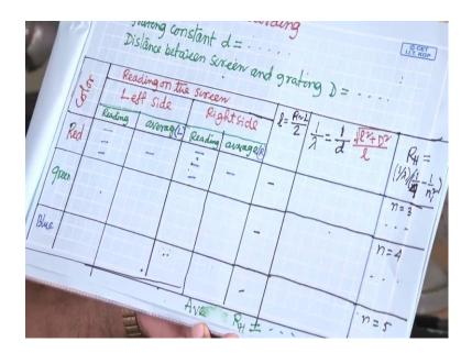
experiment of data we will record. this type of table we will use. grating element d; as I told this 600 lines per millimeter. what is the separation between the lines that you can calculate? that could be 1 by 600 in millimeters. that will be the d. that you should note it is since it is supplied. Distance between the screen and the grating that capital D whatever I showed in figure. that we should fix it we will not disturb it that you should note down.
