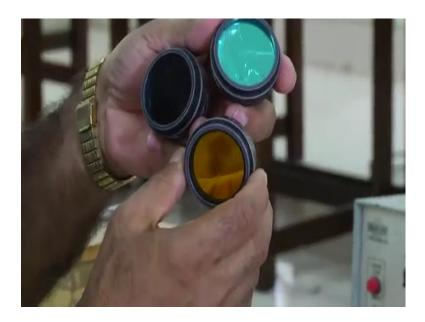
we will use this; these are interference filter. it will only allow light of wavelength 405 nanometre that is the wavelength of light we will pass through this filter and other light will be stopped.
