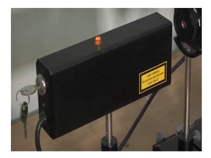
this is the laser source, this is the laser source; generally, laser source gives the monochromatic light, and also parallel light; also, parallel light, but there is a divergence of this light.
