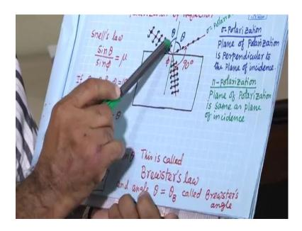
from Snell's law actually sin theta by sin phi this is the refracted angle equal to mu refractive index of this glass, Now, in this condition; under this condition at Brewster's angle we can write this theta plus 90 degree plus phi equal to 180 degree; equal to 180 degree theta plus phi theta plus phi is 90 degree phi equal to 90 degree minus theta. sin phi equal to cos theta, here sin phi we can replace with the cos phi cos theta. mean equal to sin theta by cos theta equal to tan theta.
