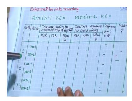
for that we will use table; we will use table find; we have to find out Vernier constant to Vernier's are there in spectrometer you know. Vernier 1 and Vernier 2; we have to note down generally both are having the same vernier constant note down the vernier constant. Then your serial number means number of observation 1, 2, 3,
