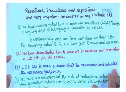
We have demonstrated how to measure resistance, basically high resistance through charging and discharging a capacitor in CR circuit or RC circuit. This experiment we have demonstrated and experimentally one can find out time constant that is RC.
