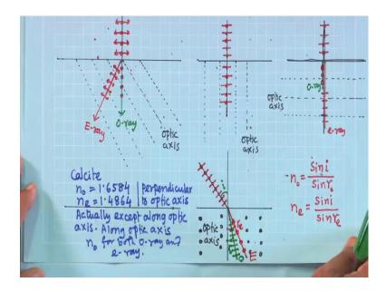
for calcite crystal what is the; what is the property? for calcite crystal this refractive index for o-ray is greater than the refractive index of e-ray, and so, this value since along the optics axis O-ray and E-ray are same their refractive index velocity is same. refractive whatever we are talking here, so definitely that is this value is perpendicular to the optics axis, all.
