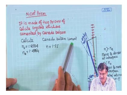
if I continue as I told this concept we use for device. prism is a device, optical device type, so Nicol prism. Nicol prism it is made of two prisms of calcite crystals, these are device; prism is called Nicol prism. it is made of two prisms of calcite crystals which are cemented by Canada balsam cement, ok, Canada balsam cement. Means cement means you can attach two object.
