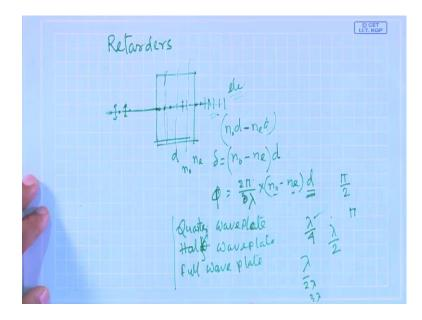
what we have seen? This when. What we have seen? When this is the crystal light is falling this way, unpolarized light, unpolarized light and. if this if optics axis is parallel to the surface, optics axis is parallel to the surface this is the direction when light is moving, so e-ray is moving faster e-ray is moving faster than the o-ray that is what we have seen, this is used.
