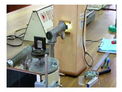
Now, I will show the experiment, so this is the experimental setup for diffraction grating. here this already we have set, and I will show you first the spectra, this is a mercury source, and this is the spectrometer. this collimator is giving us the parallel rays because we have set for parallel rays using the Struthers method and this is the grating this part is grating. light is coming falling on the grating, so we set it for normal condition,
