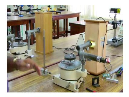
Then from this whatever reading it is a approximately I can tell you, so this is around I can see 90, then I will add with this reading 90 and then at that place I will set. it should be around 180 or 0 yes; it is 0, it is around 0, so take this reading telescope is rotated through 90 degree and set at angle, so it 0 for this vernier. another Vernier you have to note down it should be 180.
