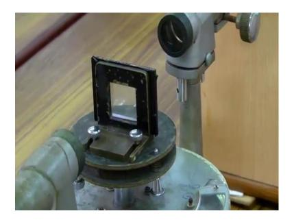
now light is falling normally on it, normally on this grating and then it is refracted different colors will be diffracted for different order.
