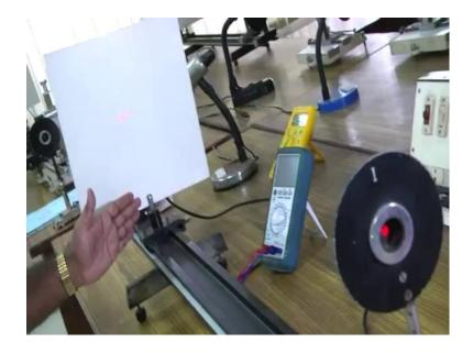
laser beam is falling on the slit, now here this is a screen, here this is a screen. we are seeing the diffraction pattern. we are seeing the diffraction pattern. this is the central one highest intensity diagram you have seen, in the diagram you have seen the central one will be highest intensity, central one will be highest intensity. And, then this side one, the secondary one that intensity will decrease and between this maxima there are minima
