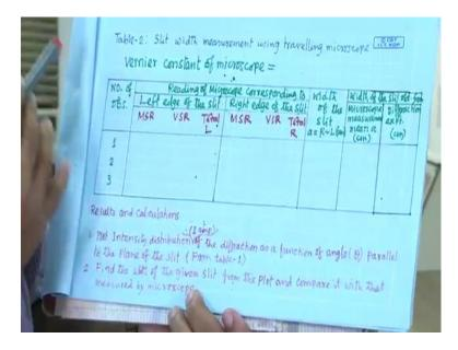
And, then the we will measure slit width using the travelling microscope for comparison whatever the experimental we have measured from diffraction experiment. we will verify using the travelling microscope. we will note down the Vernier constant of the microscope and then we will take reading of microscope corresponding to left edge of the slit, main scale reading, Vernier scale reading total.
