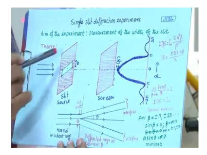
today I will demonstrate a Single Slit Diffraction experiment. aim of this experiment is measurement of the width of the slit. we have a slit single slit, its width is b. So now, parallel rays are falling normally on the slit this red part is opaque and this rectangular part is open. light will pass through this slit and after passing through the slit, if slit width is its width is in the order of the wavelength of this light; then we will see the diffraction pattern on the screen.
