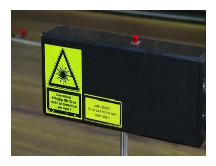
its wavelength is as I told 632.8 nano meter. this laser beam is falling on the slit.
