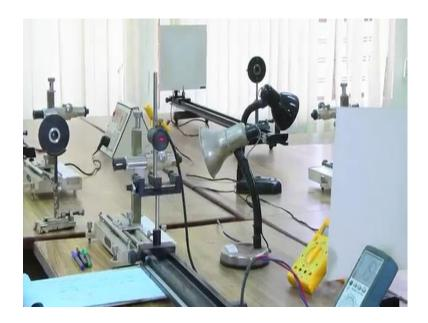
Now, I will remove the screen. this is the photocell So now, that diffraction pattern is falling on the photocell. photocell will give photo current or photo voltage
