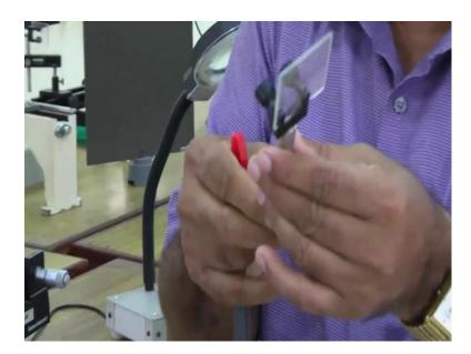
these we have inserted this you can see this in middle so there is a line. that is the age of this biprism these biprism we have inserted we have inserted in one of them, so this is one mirror this is another mirror so light is coming from this glass plate so in this direction in this arm I have put this biprism and these biprism is on a translational stage, this translational stage it has linear scale as well as Vernier scale.
