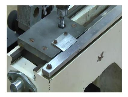
Vernier scale have these 50 division and linear scale it has smallest division is 0.5 millimetre, so you have to note down the least count you have to note down the least count for so these the table.
