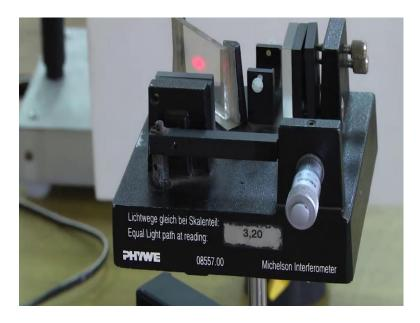
this is the micrometre this is the micrometre is like it is like screw gauge this micrometres so initial reading we have to take initial reading is here, I can see this is a initial reading this circular scale that linear scale reading, I can see these 6 6 5.5 it is a 5.5 millimetre and this circular scale reading is it is a almost is 0; almost it is 0 least count we have to find out.
