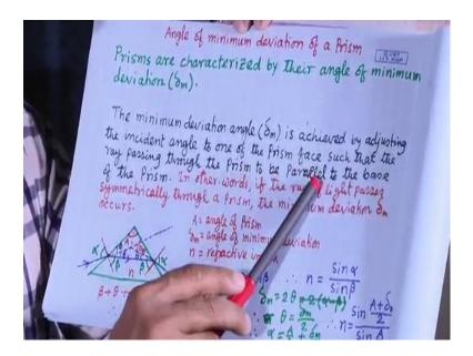
now another important characteristics of prism is the angle of minimum deviation. prism is characterised by their angle of minimum deviation. the minimum deviation angle is achieved by adjusting the incident angle to one of the prism face such that, the ray passing through the prism to be parallel to the base of the prism.
