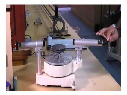
this simple method what is that let me take it out. first what we have to do for parallel rays. here eye piece is set at the distance from the cross wire in such a way that cross wire is focused; that means, cross wire is at the focal point of the eye piece.
