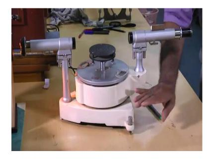
before experiment we have to make sure that vertical axis of rotation and the horizontal axis of the telescope and collimator, they are perfectly positioned
