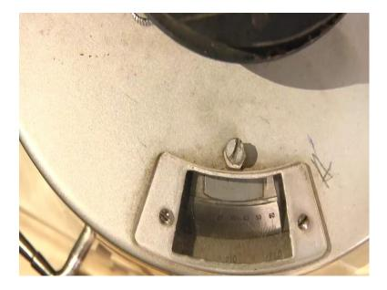
here if I show you, I think it is a; I can show you here. this is a let see this main scale; main circular scale is attest with the telescope; attest with the telescope, if I move this telescope; that means, this main scale, main circular scale is rotating, and vernier scale is attest with the prism table. if I rotate the prism table, you're this Vernier scale is rotated,
