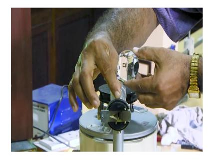
you know this convex lens; now, there is a convex lens, and this is the source. Now, if I put this source at the focal point of these lens then we will get other side, we will get parallel rays, this we move, this we move to put this source at the focal point of the lens inside this tube, collimator is make of it has two part, one is lens convex lens it is fixed inside of this tube and it had source, to get the parallel rays we have to put this source at the focal point of the source.
