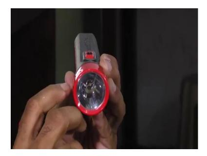
You have a bulb here, inside you have bulb, and surrounding this bulb we can see this the, it is the mirror, it is the concave mirror, concave mirror we are using concave mirror. this light on the bulb, it will go this all side, now this concave mirror inside it is there it will reflect this all this light and converge towards outside, you will get more light from the same bulb. in torch light, we use the concave mirror, ok, so that is what here one can see.
