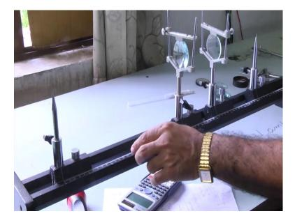
now I got the suitable position. if I keep the convex lens; if I keep the convex lens out of 2 f. it is f is say around 10 for this convex lens. if I keep it; so, 2 f is 20, so if I keep away from the 30. I kept it at around 30 and then so; that means, the image I will get within f and 2 f within f and 2 f.
