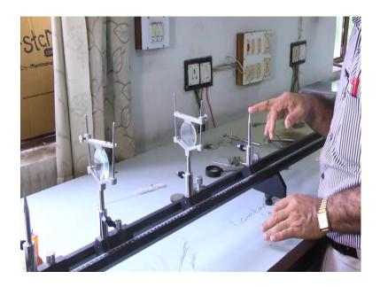
Now, I will put this is the; this is the concave lens we want to measure the focal length of this concave lens. now, I will put this concave lens between the image needle and the convex lens. let me fix it and then let me keep at a particular distance say I will keep at it is at 15.
