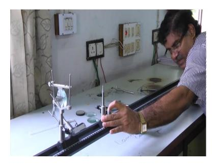
If I remove this one; so I have to I will find out the image position and it will be closer to the lens; it will be closer to the lens because now object distance is more than 2 f. image distance will be within if f and 2 f this is the other side. now in this way actually image I am getting closer to the closer to the than the earlier distance earlier it was greater than 2 f, it was greater than 2 f yes. it's around I can say yes.
