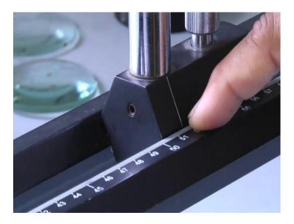
It's around say 51.8. this is the now this is the position of the image needle for this convex lens for this position when it is at 30. now, I will not disturb these two. this
