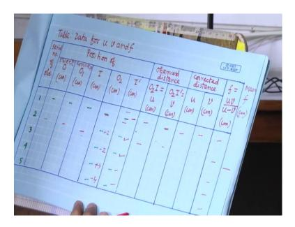
Unit table data for u v and you can find out f. number of observation and then position of O means this in this case O I have I have mention this is the object O means here object position, O 1 optical center of the lens which lens this is the convex lens O 2 is the this concave lens and I is the image of this lens convex lens and this is the image for the when you are putting this O 2.
