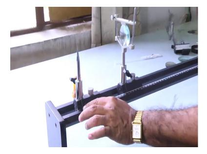
here same lens convex lens we are using say its focal length is around 10 to 12.
