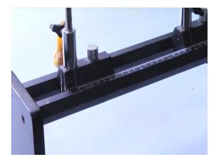
This is the same optical bench this is the same optical bench it has it has meter scale meter scale. 0 to 0 to 150 centimeters 150 centimeters.
