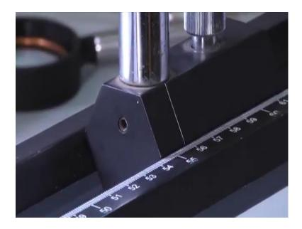
Needle image it is 55 point; I can see 55.8; ok point 8as I told this is not the unique position. one should again one should again try to find out the better position take 3-4 observation take 2-3 observation now it is 55 point I can see 4; 55.4. take three observation and then find out the average of that one. then you will get the u and you will
