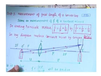
For measurement of focal length of a convex lens. this it is procedure is same as the measurement of focal length of a concave mirror. for concave mirror we have seen that or for mirror formula actually in working principle the mirror formula we have used that is 1 by f equal to 1 by u plus 1 by v right or 1 by v plus 1 by u.
