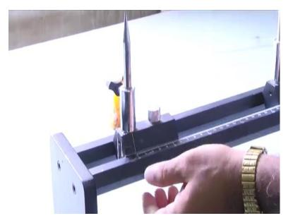
And this is the object needle. I fix that object needle at 0. index mark is coincide with the 0. let it be fixed and then these lens I have seen I think I will not repeat that one, but or I can do that.
