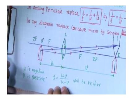
This lens produces the image whether it will be virtual image, or it will be real image, that depends on the distance of the object from the mirror.
