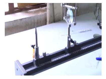
I will keep object distance from the lens is 1.5 times. say let me keep this then I have to keep this lens is say 15 if it is 10 or 12. let me keep it at say 17. focal length is 10. it is 20 2F is 20. I am keeping the object distance 1.5 times more or less.
