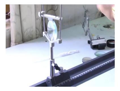
Now, this one is convex lens. we put convex lens in a holder, lens holder and that we that holder we put on the upright. upright; that we can change the position of this it can move from the optical table optical bench.
