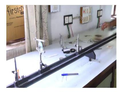
Now, I have to take this image needle, I have to take the image needle and first what I have to do? I have to change the distance and first that inverted image tip and the object this image needle tip should coincide.
