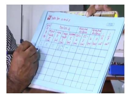
You need table to record, the data you need table to record the data. data for and u and v. here serial number of observation position of object needle, then lens, then image needle as I told image needle you take three observation then find out the average of that image reading. now, object distance is u and v O dash OO dash and O I that is v.
