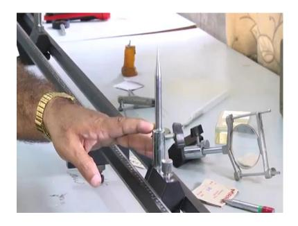
And another needle I need to get the position of the image, so this the image needle.
