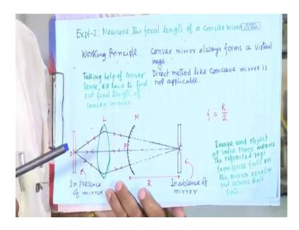
That is the experiment so remember these sequence first without mirror I must find out the position of the image due to the lens. And then I will put lens and mirrors, concave mirror, convex mirror and I will try to find out the position of the mirrors to get the image on top of it. unfortunately, in camera I cannot show this, this co-incidence and this parallax method, but I will show the step how to do the experiment. this is the same optical table as last time we have used.
