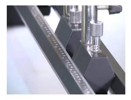
Now, I must go other way slightly. Now, it is nice, so there is no parallax. now I must note down the; I must note down the position of the position of the mirror. It is the around it is a 6 the 62, it is a 62. P I so difference between these two this 62 and this 106 or 107 approximately, 107 and 62 so how much you are getting, 4 45, so this P I is 45, P I is 45.
