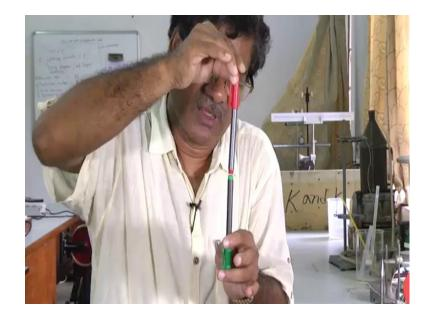
One has to; one has to remove; one has to remove the parallax; that means, first what you have to do this here you have image needle say and then image real virtual image you have to see through the mirror or the lens and you have to change the position of the image needle and try to find out the position, so that this image tip will come on the tip of the needle image needle.
