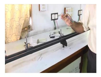
Change the position of the object by 2.5 centimeter. And for each position you, you find out the; you find out the position of the image needle. How to find out that I explained you, so for each you object distance, you must find out the image distance following the method as I described. we will get data for different u, you will get data for different v.
