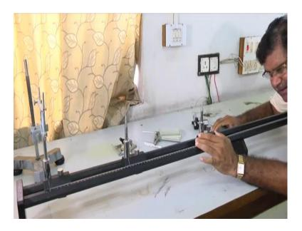
Now, I will set my eye in such a way, so this tip of this needle image needle and the tip of the tip of the image, they are on the same line. Now, what I must do is the parallax method. I will close my left eye and open my right eye and I move my; I move my head left and right and I must see that this both tip at which for which position of the needle, object needle this image needle.
