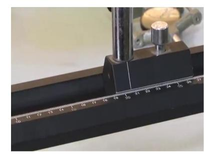
When reading is around yes, around 20 also. it is approximately this focal length of this mirror will be around 20, so plus minus some this is just this is approximate. I must keep the keep the distance, I have to keep the distance of the object will keep between f and 2f means, between a focal point and the at the point of ready centre of curvature 2f c.
