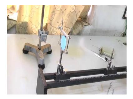
What is the procedure for doing experiment? take a mirror concave mirror for measuring the focal length of that mirror, so you must so these the holder of the mirror, so you have to fixed hold these mirrors. Now, this mirror is so we tell this is the upright, so it is a this is the ok; this is the holder of mirror this is on part and this we tell this upright.
