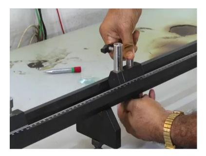
If I want to fix that the particular position, so here I want to fix it. I pressed it and then rotate it ok; so now you cannot move; now you cannot move. if you want to move, just release it and it will move.
