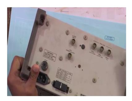
This tube end is basically the display. And this other end of the tube you see other end of the tube is just which it is a, this the back side panel. So, here you see this the power with power cord, we give power 220 volt and here some something, whether you are using
