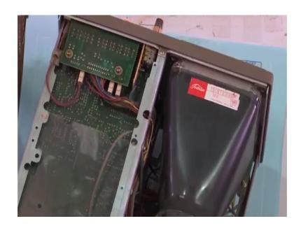
So, this is the front panel ok, I have shown you, this is the front panel. So, now I have opened it, when I opened it I can see this half of the portion of this, inside of this one is one tube ok. So, this tube is called the CRT Cathode Ray Tube, and it is basically is a it is basically with display.
