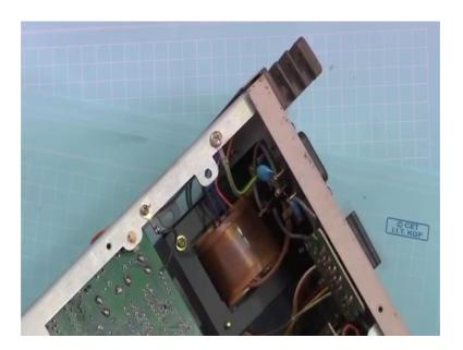
So, these one, this one is transformer. Now, in this for running for operating this CRO, we need very high voltage for CRT – Cathode Ray Tube ok. And for other component, this other control, horizontal control, vertical control, triggering so you need normal
