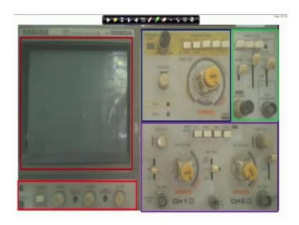
So, if you see the front panel of this CRO front panels of the CRO, so I can tell this is a front panel is basically arranged in a in four blocks. So, this I mark with a red color. So, this is a display, this is a display and display control, these knobs are basically to control the display on the screen whatever we will display on the screen, so that will be controlled by this four knob. So, I will tell what are those things.
