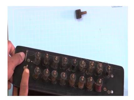
But opposite side of this resistance box this top part is if you just rotate it. So, what you are seeing? You are seeing just this; you see these are this wire threaded right here very thin wire. So, this it is we have rounded it on a some insulating wheelers.
