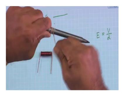
So, here I will show you so, you see this is the wire; this is the simple wire this is the simple wire; this is the simple wire. Now from there I can if I want to make inductor so, just it is simple by definition ok; you just roll it.
