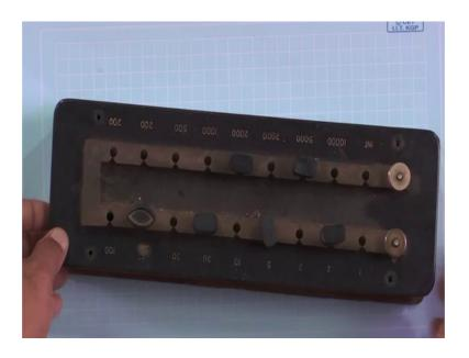
So, basically from on left so this resistance box and all of you have seen in laboratory. So, this resistance box here it is a resistance is a 1, 2 then 5, 10 right the up to it is the one it is a 10000 ohm. So, these 2 are thus in connection; so we with we connect these 2 in our circuit. So, when we connect this 2 in our circuit. So, this is the resistance included in the circuit.
