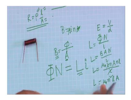
What is i? Is current passing through this coil what is n? N is number of transfer unit length; number of transfer because it is infinitely long is very long solenoid. So, n is number of transfer unit length of the solenoid and A is the; A is the area A is the area of this of this coil; so, this will be give you magnetic field.
