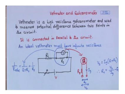
So, voltmeter is a high resistance galvanometer and used to measure resistance difference between two points in the circuit right. So, it is connected in parallel to the circuit.
