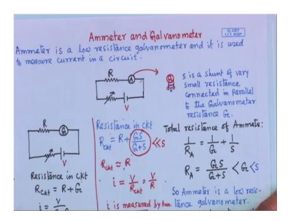
So, ammeter is nothing, but galvanometer, it is a low resistance galvanometer ammeter is a low resistance galvanometer and it is used to measure current in a circuit ok. And this
