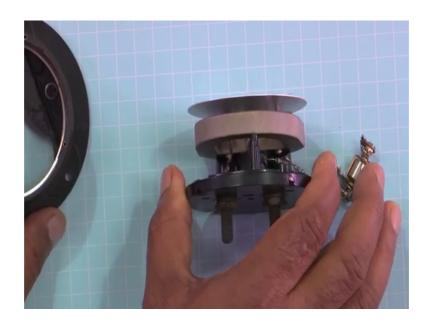
So, voltmeter is basically a galvanometer of high resistance. So, what is the galvanometer volt voltmeter? So, voltmeter is basically a galvanometer; voltmeter is basically a here I just I have shown you.
