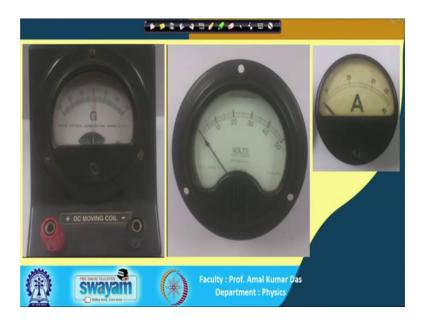
So, I was showing you these three main tools a apparatus, we use in our laboratory when you do electrical circuit. So, these are the common tools common apparatus we use, and I was discussing about the galvanometer ok. So, today I will discuss about the voltmeter and ammeter.
