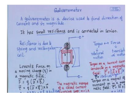
So, galvanometer is basically a galvanometer is a device used to find the direction of current and its magnitude. So, direction of the current and its the magnitude of the current, that is the we determine we find out from the galvanometer ok.
