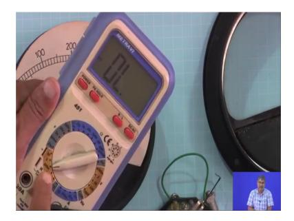
So, if you want to measure voltage, if you want to measure even frequency one can measure ac voltage also one can measure and you can measure the capacitance in this f is written capacitance f is written it can measure capacitance it can measure h means henry inductor inductance you can measure inductance capacitance resistance you can measure using this one even you can measure this check this np np np transistor also.
