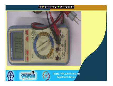
So nowadays, so we have very good multimeter. So, multimeter is basically it is voltmeter and ammeter and some more things you can measure direct resistance and you can measure directly the current flowing through the through the through the circuit ok. And also many more things you can measure you can check this here you can see this you can check this.
