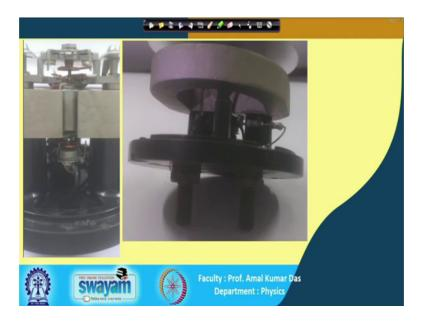
So, I think here its a looks better, here its looks better. So, here also you can see this is the galvanometer structure and with this galvanometer structure that spring here also we can see in better with one spring up and one spring down, and then I think this is the this is the coil this is the coil rectangular coil.
