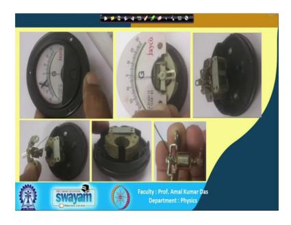
So, I think in figure here its more clear here just check it. So, I have taken picture. So, this is the rectangular coil; this is one spring, this is one spring, and this is another spring
