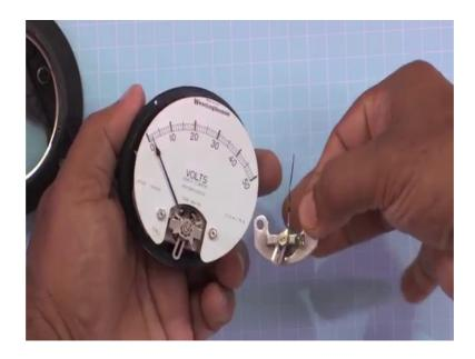
If I open it; so here I have not opened completely, so this here this part you are seeing as the same as this one you know already I have opened, this part is same as this one you can see. That means, this galvanometer this is the galvanometer main part of the galvanometer rectangular coil etcetera. So, that is there.
