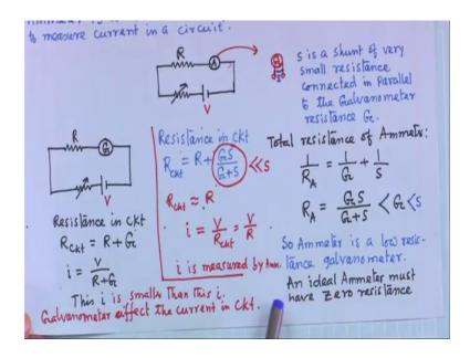
Actually this resistance in ideal case and in ideal ammeter this resistance generally its taken as a zero resistance or tends to zero resistance. So, why we need why we need to make it smaller resistance zero resistance or very very small resistance; because in my circuit current is flowing and that current I want to measure for that I am using an instrument that is called ammeter. So, that ammeter I am connecting in a series in the in series of the circuit.
