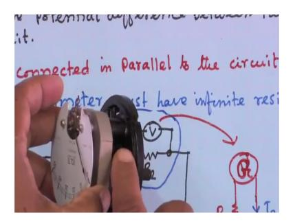
So, additional resistance this Rv I have written. So, that is the basically additional resistance of this is R v and g is the resistance of the galvanometer. So, here you can see here you can see this 1 by g plus Rv that is the resistance of the voltmeter and 1 by R 2 ok.
