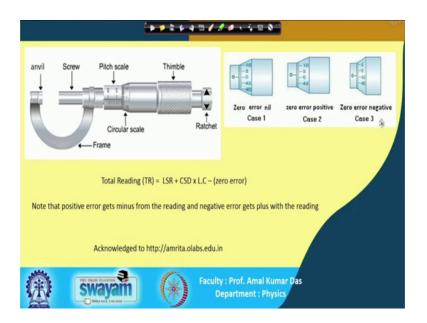
So, in screw gauge about zero error: so in this case it is a negative zero error, because it just cross this zero of the linear scale right.
