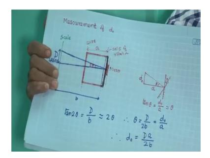
So, that I will basically tell you, that measurement of D measurement of D. So, you see. So, this upper part I have drawn upper part I have drawn, upper part this I have drawn. So, here mirror is here, mirror is here. So, and I put weight here I put weight here and then you touch this bottom wire. So, when it touch this bottom wire; that means, it is rotate, and then mirror also rotate.
