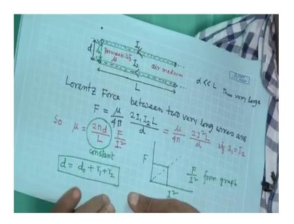
So, what is left in our formula working formula what was there is a mu equal to 2 pi d capital L divided by capital L f by I square. So, this d I have measured this d I have measured r 1, r 2 as I showed from using slide not slide calipers using screw gauge and d 0 using this optical method. This is you tell light mirror arrangement light mirror or light lens scale arrangement. So, from here view as able to measure the measure the d whatever we need in our working formula.
