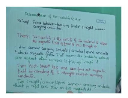
So, this you know this permeability is the ability of the material to allow the magnetic lines of force to pass through it to pass through it. So, to determine this permeability here method we will use that is basically force between 2 long parallel straight current carrying conductor.
