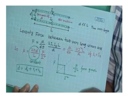
So, this the fundamental basic concept of producing magnetic field in a current carrying conductor. So, basically we use the biot savarts law to find out the magnetic field. So, here so, this a conductor it is a length say it is L and current is flowing this 2 conductors. So, they are separated they are this distance is d ok. So, this centre to centre this axis of this wire and this of the other wire.
