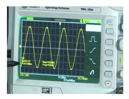
So, now here it is the take reading for 0 position take reading this for 0 position this is the here is it is giving reading ok, it is the V pp 6.15 volt. It is giving 6 point I can see properly, yes I think 6.20, it is changing. So, let me write 6.20. So, for 0 angle. Now, this for this 6.20 ok.
