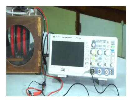
So, there will be induced emf on the secondary coil, so that induced emf ok, so we will we will we will so this is the these two are from this secondary coil. So, this induced emf ok, this voltage we have put in this oscilloscope this is oscilloscope. So, from this oscilloscope, I will know this voltage induced voltage whatever generated in secondary coil, so that voltages reading I will get from this oscilloscope ok.
