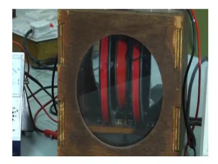
So, here you see this whatever coil I show, this here two coils are kept bigger coils two coil circuit. This we are telling the primary coil ok. We could do the experiment with one coil ok, but here just two coils we kept that two just to increase the magnetic field. So, it will be just double, and then your signal will be higher.
