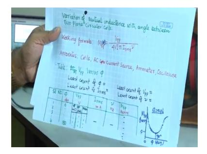
So, now basically reading this setup, we are going to study we are going to study the variation of mutual inductance with angle between two plane circular coils between two plane circular coils. So, there is the experiment, we are going to demonstrate now. And working formula for that is basically M as a function of phi, sp because is just to represent primary or secondary coil, people write 1 2 M 1 2 etcetera, so that equal to this V pp by whole square root of 2 by I rms nu ok.
