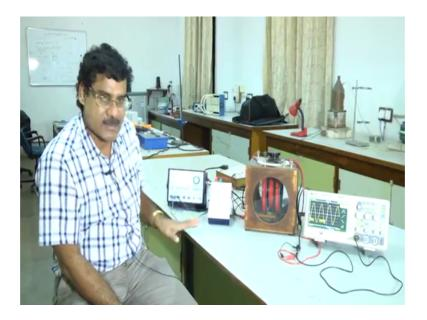
So, let me just show you the experimental setup first experimental setup first. So, this is the experimental setup for studying the mutual inductance ok.
