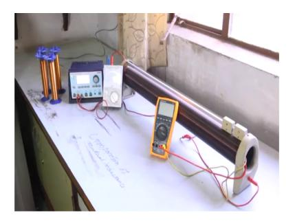
So, here this is this very simple experimental setup for this experiment. So, as I told that in this setup what are the apparatus we require? We need one solenoid. So, this is a solenoid this is a solenoid, you see the number of turns, it has many number of turns ok; so, this is the solenoid.
