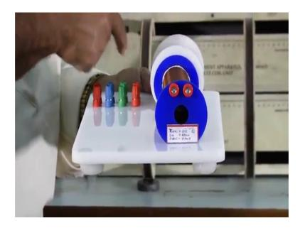
Now, here is a an inductor, it is a basically a PVC pipe. On the PVC pipe, we are winding of insulated enable insulated copper wire. Now, see here I made already 30 to 40 turns, none increasing the number turns. This type of wires are available in market in various gauges. According to the according to your (Refer Time: 11:58). I mean current in the coil current in the circuit you select the gauge of this wire.
