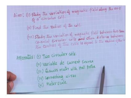
So, aim of this experiment is to study the variation of magnetic field along the axis, along the axis of a circular coil. Then find out the radius of the circular coil, then study the variation of magnetic field between two same coaxial circular coils a basically Helmholtz coils, when distance between the centers of the circular coils is equal to the radius of the coils ok, so that is what we want to study in a in an experiment.
