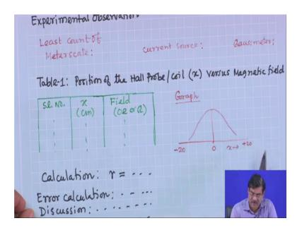
And there what we have to do we have to, so you have to note down the experimental observation. First as I always tells, you have to you have to find out the least count of your apparatus, so that is the least count of meter scale you have to write, current source for current source what is the least count, for gauss meter what is the least count that you have to noted down.
